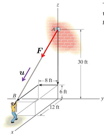
The force vector  $\boldsymbol{F}$  acting a long the rope can be defined by the unit vector  $\boldsymbol{u}$  (defined the <u>direction</u> of the rope) and the <u>magnitude</u> of the force.
