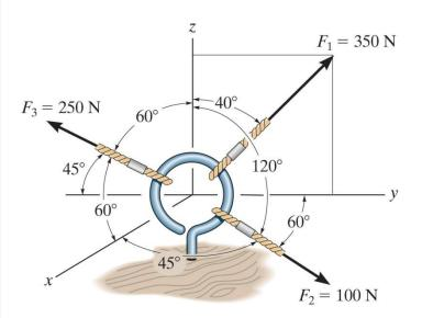
The cables attached to the screw eye are subjected to the three forces shown.
